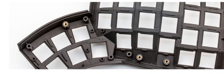
Glove80 has an exact and complex 3D form which we were able to realise with only two pieces of plastic. To make this possible, the tooling required carefully designed non-parallel parting planes to eliminate undercuts. This was particularly challenging because the hole for every switch is pointing in a different direction, which required cleverly designed cut-outs around each hole to avoid undercuts. We were able to create moulds with only one side action (for the USB connector panel).
