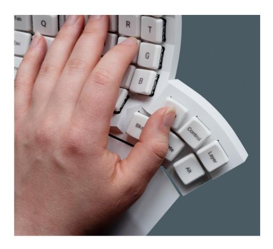
We also developed the thumb key arrangement through extensive testing. Thumbs are the strongest digit of the hand, and are remarkably underused when typing on a standard keyboard. Several contoured keyboards have thumb keys arranged in a cluster. However, none are designed around natural thumb movements, and typically require users to move their palms to reach some of the keys.
